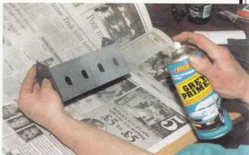
Applying a thin layer of undercoat
