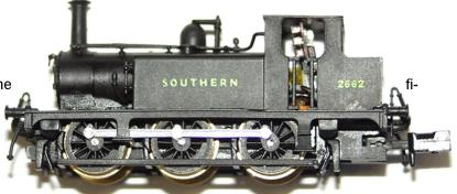
The motor gears should be checked for correct meshing, and the pickup strips remain positioned on the inside of the wheel rims.
