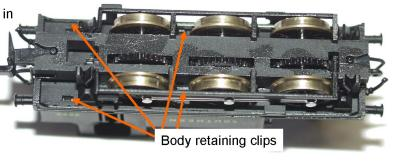
The motor is held in place by mouldings in the upper body, and soldered to a pair of brass strips, which are also the pickups, once the upper body is removed,
